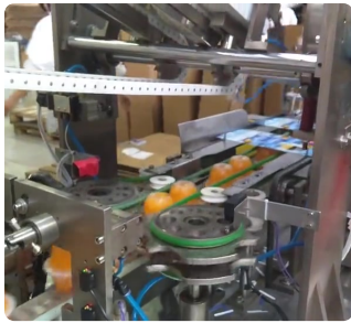
Rotating aligners orient the cups
